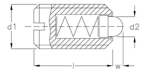
$\begin{array}{ll} \text{d1} & = \text{M16} \\ \text{d2} & = 8.5 \\ \text{Length I} & = 24 \\ \text{Spring pressure N bottom} = 100.0 \\ \text{Spring pressure N top} & = 50.0 \\ \text{W} & = 4.5 \end{array}$
